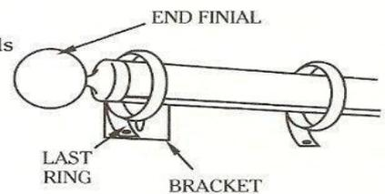
Install end brackets above and 15.2 to 45.7cm (6" to 18") to the sides of casing. Place centre support bracket equidistant between end brackets. Adjust bracket projection at screws "A".
